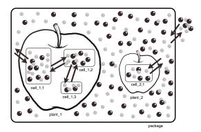
Figure 1: A schematic representation for the MAP system model. In this case, two produces share a package:  $plant_1$  is formed by three connected cells, and  $plant_2$  is formed by a single cell. Arrows represent paths for molecules (spheres) diffusions
