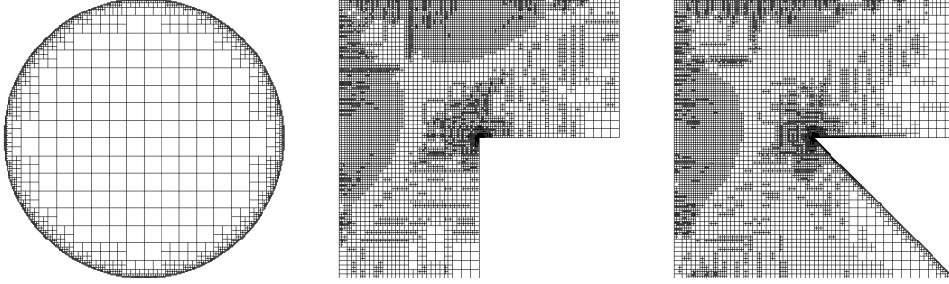
FIGURE 6. Left: Locally resolved disk, 13 875 degrees of freedom. Middle: Adaptive mesh of the L-domain, 36 798 degrees of freedom, level 17. Right: Adaptive mesh of the cusp domain, 44 793 degrees of freedom, level 20.
